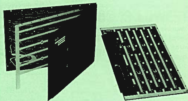
Figure 3. All Printed-Circuit Cards for the Ruggednova Use the Same Construction Techniques. This Picture Shows a Standard Printed-Circuit Card, the Heat Frame and "Cookie Sheet."
